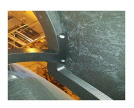
2. Remove the cover plate of the lifting loop by opening the 2 torx screws.
