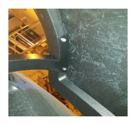
9. Align the pop rivet holes and install the rivets
