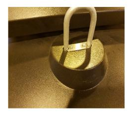
10. Install the filling lid with four screws. Use a medium thread lock and spring washer.
